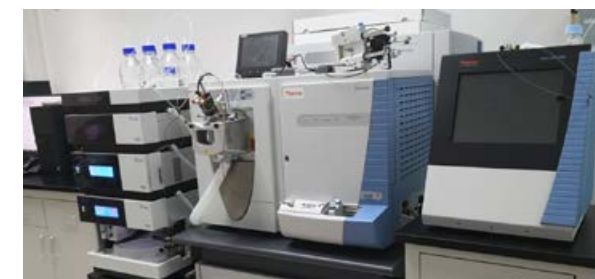
Figure 3. High resolution double pressure linear ion trap-orbitrap-liquid chromatography - mass spectrometry
